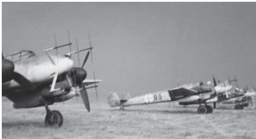
A group of Bf 110G-4 nightfighters from NJG 4, possibly at Florennes airfield, in Belgium, in mid-1944. The introduction of the improved FuG 220 Lichtenstein SN-2 radar in 1943 swung the duel back in favour of the Luftwaffe for a while. (Bundesarchiv, Bild 101-492-3347-028, Foto: Güntzel)
