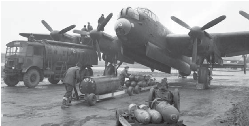
A Lancaster from No. 3 Group's No. 75 "New Zealand" Sqn is loaded with bombs at Mepal, in Cambridgeshire, prior to participating in a night raid over Germany. By 1944, Bomber Command was aware that between ten and 30 per cent of the bombs it was dropping were failing to explode due to faulty fuses. A number of Lancasters were also destroyed by their own bombs detonating prematurely. (Imperial War Museum CH 14680)
