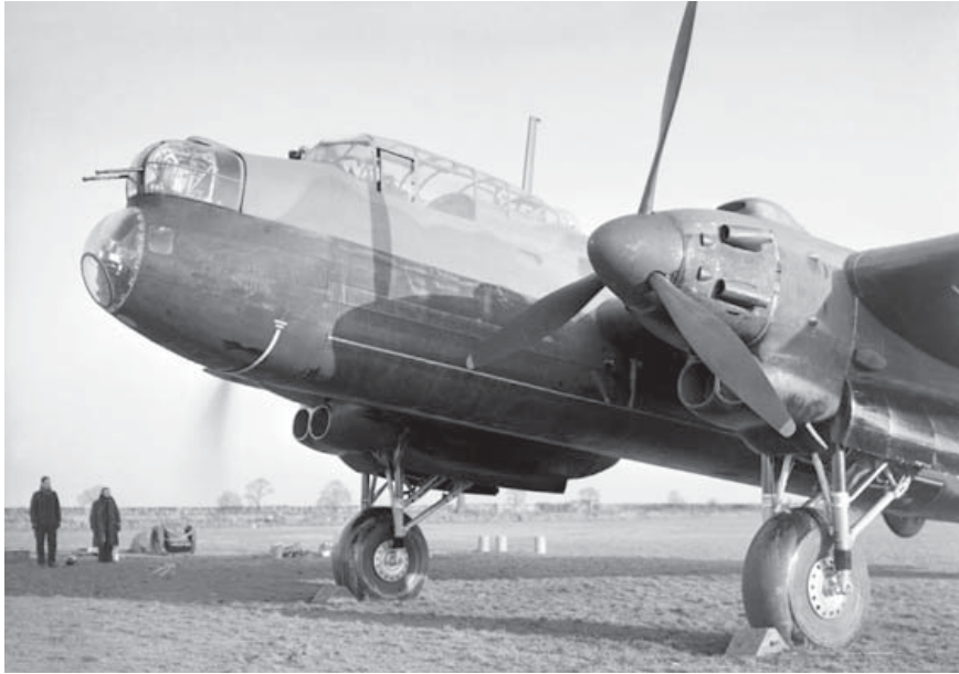
The Manchester bomber was plagued by its unreliable Rolls-Royce Vulture engines, which over-heated and had poor operational reliability. Despite Chadwick's best efforts the Manchester remained unsatisfactory, and the Lancaster was developed as a four-engined alternative. [Imperial War Museum, CH3879]
