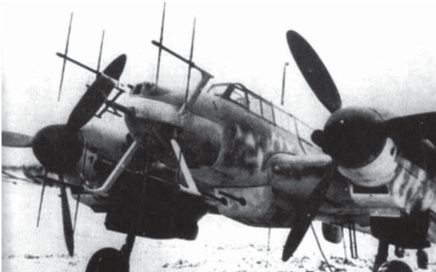
A Bf 110G-4 nightfighter with four large FuG 220B Lichtenstein SN-2b radar antennae surrounding one smaller FuG 212 Lichtenstein C-1 antenna. Many Bf 110 pilots disliked the additional weight caused by large nose-mounted antenna arrays, which cost them about 40mph in speed. Note that this aircraft also has additional 20mm cannon fitted in a centreline belly pack. (Author)
